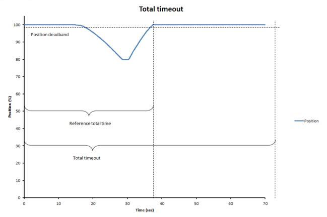
The partial stroke warning parameters are set to the following values:
