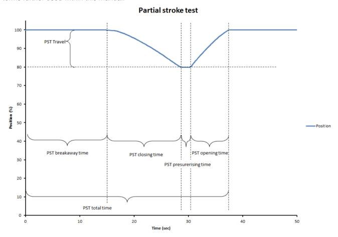
When a partial stroke is started the position is evaluated. The valve must be full open before the partial stroke can start.
