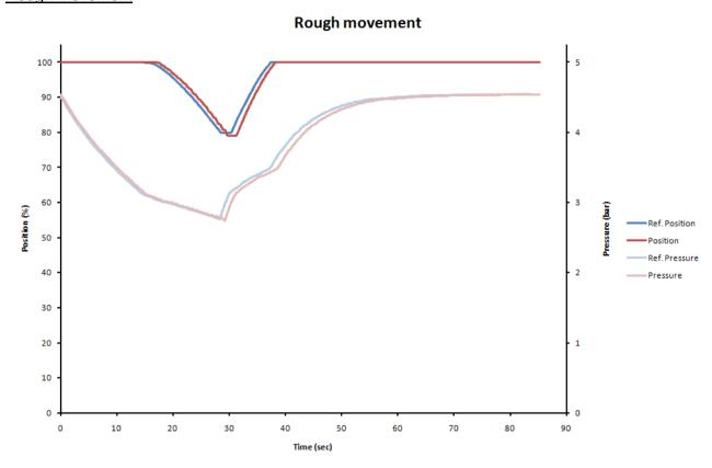
The Type VSD Controller will not report errors if the deviations from the reference curve are small. In cases like this the signatures must be extracted and analysed visually in the VCDC Software
