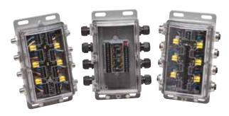
The FieldBlock platform is designed to interconnect field devices to the communication network in nonincendive, intrinsically safe, and general purpose applications. It may be used for flexible and hard conduit wiring systems. With its rugged corrosion proof enclosure, variety of drop connector, and I/O module configurations it will prove invaluable in field networking applications.
