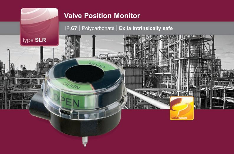
Type SLR engineered resin (polycarbonate) valve position monitor Certified ATEX II 2 GD / Ex ia IIC T4/6 provides an economical and rugged feedback system ideally suited for zone 0,1 & 2 hazardous area locations typically found in the process industries. The IP67 enclosure has a part-turn quick access cover and high visibility open / close position indicator.
