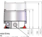
2 or 3 x Conduit Entry Size Options: Central Entries - M20, 1/2"NPT or 3/4"NPT Offset Entries - M20 or 1/2"NPT
